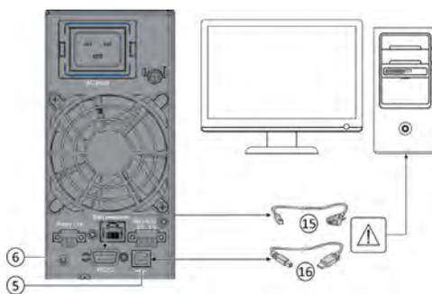
1. Connect the RS232 (15) or USB (16) communication cable to the serial or USB port on the computer equipment.
