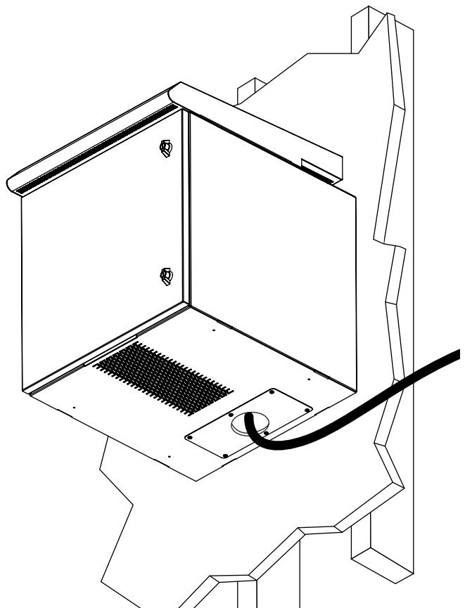
**Note:** To maintain a NEMA rating, use sealed fittings in the cutouts when connecting to conduit. Accessory gland plates with model numbers SRGP1KO, SRGP2KO, SRGP3RM and SRGP4PLASTIC are available (sold separately).
