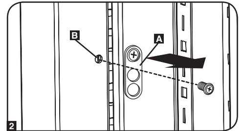
**3** Loosen the screw in each baying bracket and turn each bracket 90 degrees toward the adjoining enclosure. Align each bracket with the corresponding baying connection point on the adjoining enclosure.
