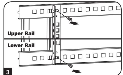
**4** Use the included silver mounting screws to secure your equipment to the rack rail. Place the cup washers between the screws and the equipment mounting brackets.
