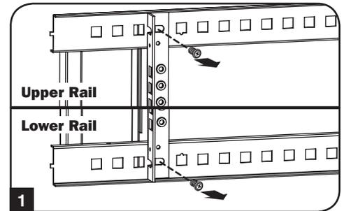
**2** Switch the rail locations. Ensure the tapped hole side of each rail is facing the front door.
