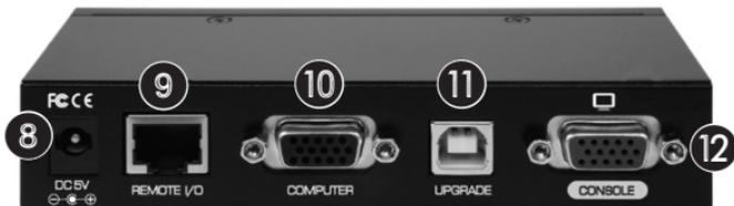
*Transmitter (TX) unit - Rear Panel*
